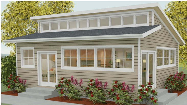
House with clerestory style roof
